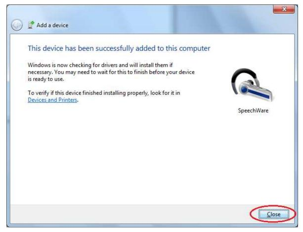
Now, your FlexyMike Bluetooth microphone is ready to be used under Windows Vista or 7! B-LED flashing twice quickly every 2 sec. means the device is on and paired with the computer but not connected.
