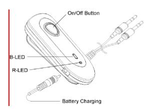
Our models **FMK03** (http://www.speechware.be/en/verArticulo.php?id=1671) --and **FMK04--** feature a couple of Light Emitting Diodes (LEDs), which lights up in Blue (**B-LED**) and Red (**R-LED**) colour, with the following meaning:
